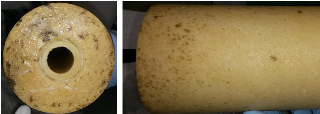
Figure 10: Biofouling in a filter cartridge (photos: Florencia Saravia)
