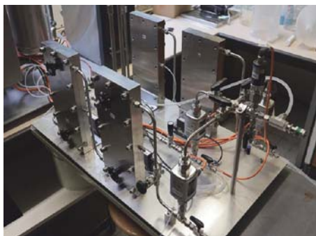
OCT image of the biofilm growing on the feed spacer (left). Photograph of the membrane set-up used to concentrate the solution (right).
