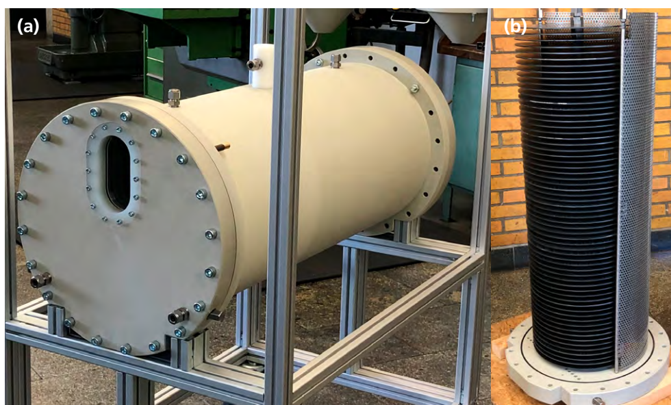
Rotating disc bioelectrochemical reactor (RDBER) (a) and arrangement of electrodes (b).
